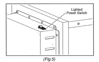
3. Check the interior rear of warmer to ensure that it is heating. The internal thermostat is factory preset to 180° F. The blower fan circulates heated air through the perforated removable chip tray located at the bottom of the interior of the cabinet (under the chips.)
